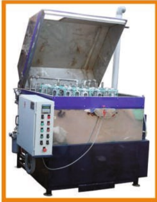
Washing facility for machinad components Millipore Testing Machine
